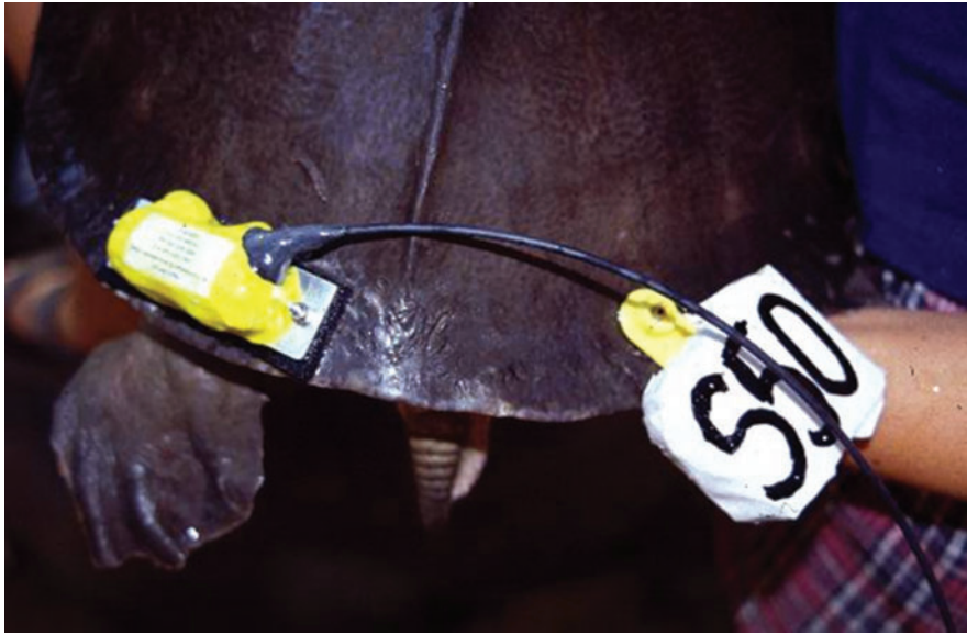
Fig. 1. Adult pig-nosed turtle ( Carettochelys insculpta ) showing a radio transmitter attached to the rear carapacial edge (left). The transmitter is ~6 cm long.
