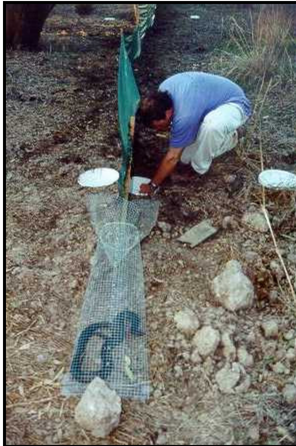
Figure 2. Photograph of a red-bellied black snake ( Pseudechis porphyriacus ) in a funnel trap employed at the end of a pitfall fence designed to capture small reptiles, amphibians, and mammals.
